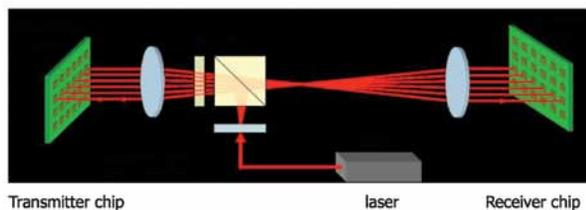
Figure 2: Parallel optical chip-to-chip interconnection over free space, with optical devices flip-chip bonded to CMOS chips.
