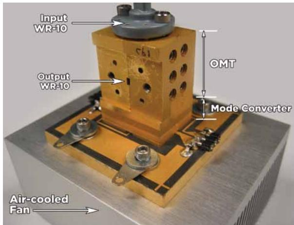
Figure 2: Grid amplifier operating at 79 GHz with an output power of 260 mW<sup>6</sup>.
