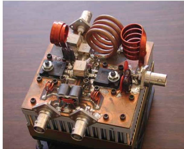
Figure 1: Prototype E/F switching amplifier developed by Scott Kee and Ichiro Aoki<sup>1</sup>. This amplifier produced 1.1 kW at 7 MHz with 85% efficiency.
