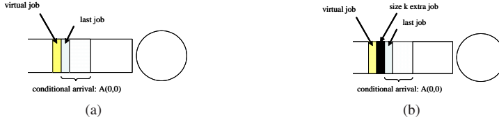
Fig. 4 Depiction of the queue state considered for the analysis of the (a) lower bound and (b) upper bound of SMART-LD.
